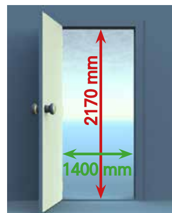
Minimum sizes of the doors / passages
